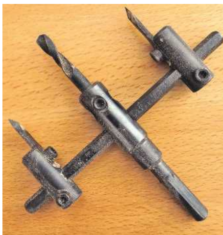
▲ Pic.9 How to cut the quadrants on the leg components? Richard uses something like this to good effect but Edward was apprehensive and rightly so. "Maybe my drill spins too fast. No matter how hard I wrenched off the grub screws, vibration worked them loose. As it whirled round the tool became terrifying, threatening at any moment to fly free and disembowel us. I think I might hide it"
